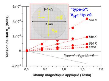
Measurements of Hall voltages as a function of the applied magnetic field at 520 K, 550 K, 580 K, and 610 K, demonstrating "p-type" conduction. The inset shows the 2-inch pseudo-substrate of transparent -Ga2O3 and the geometry of the measurement: current j, applied magnetic field B, and Hall voltage VH.
