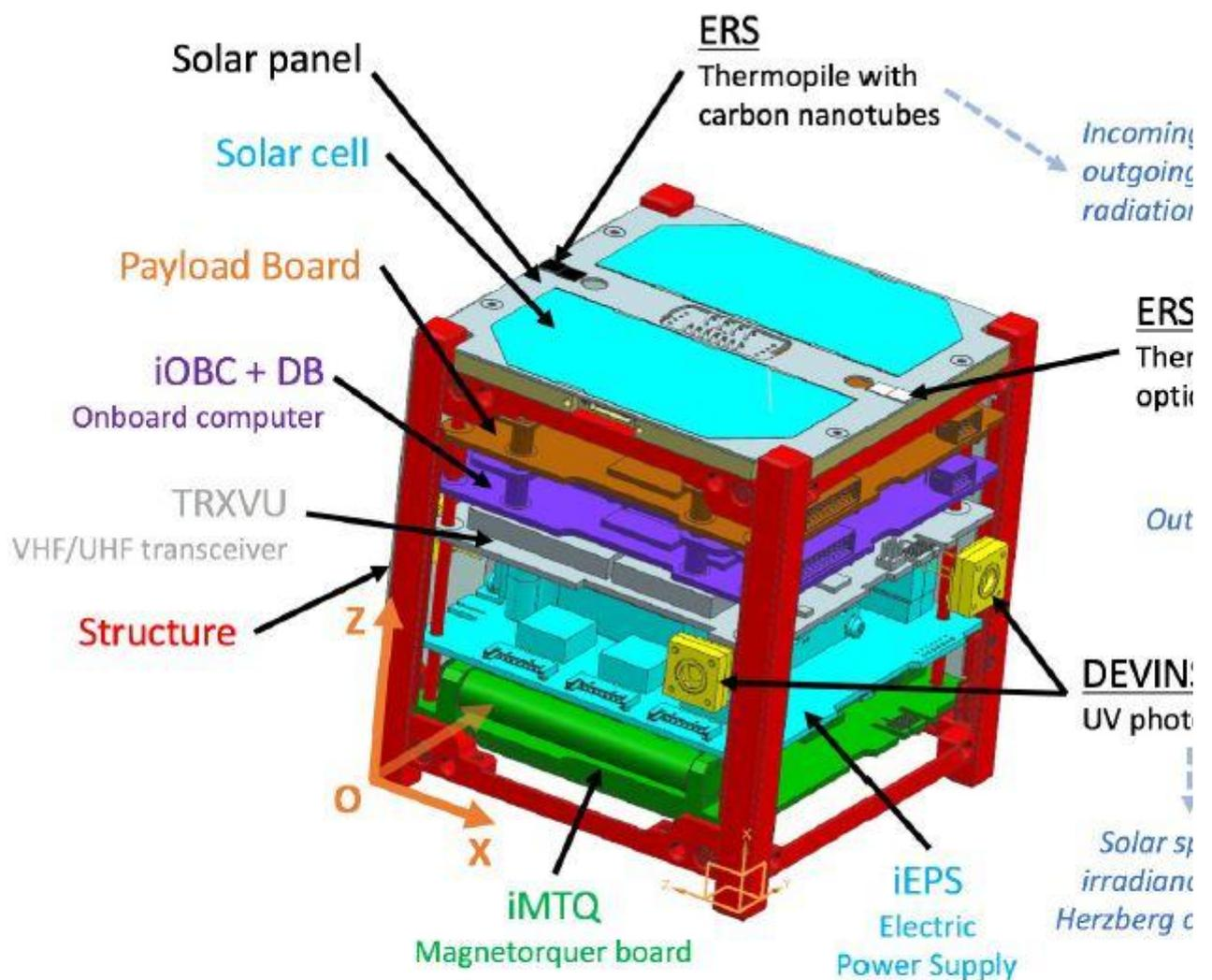
**Figure 2.** UVSQ-SAT computer aided design representation with an arrangement of Boards (PCBs). The UVSQ-SAT payload instruments are shown (Earth Radiation Spectrometers (ERS), Deep uV Innovative detector technologies for Space observations (DEVINS), accelerometer/gyroscope/compass, which is located above the payload electronics).
